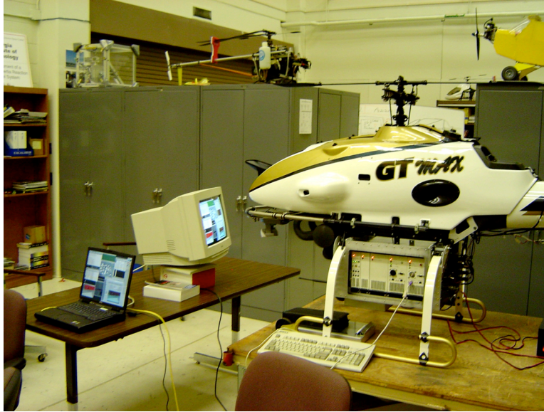
Fig. 12 Simulated and recorded-actual images presented to the image processing and mission management subsystems in laboratory testing (camera under nose of helicopter has lower right of white computer monitor in view)
